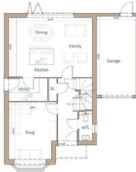
Proposed Ground Floor Plan Scale 1:50
