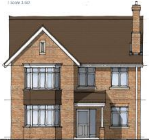
Proposed Front Elevation Scale 1:50
